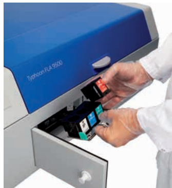
Fig 2. Filters are easily exchanged by the user.
